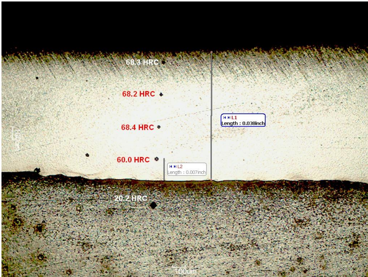
A typical cross section photo (50x) of a process qualification sample for ASME Section IX. Base material is SA-213-T22. Photo shows good overlay density, no cracking, no Lack of Fusion (LOF), very low dilution and minimal HAZ.
